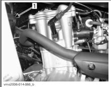
LH SIDE OF ENGINE 1. Air injection valve
